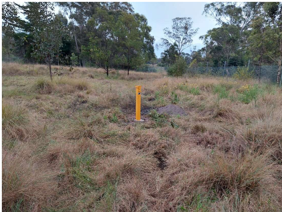
Photo 10 : Typical piezometer installation process
