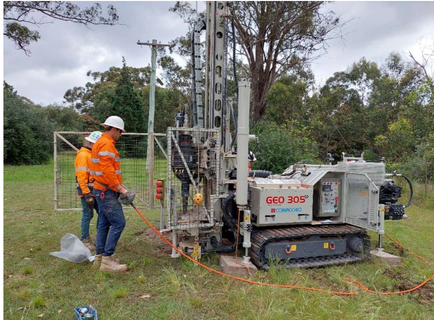
Photo 9 : 5.5t track mounted drill rig typical setup
